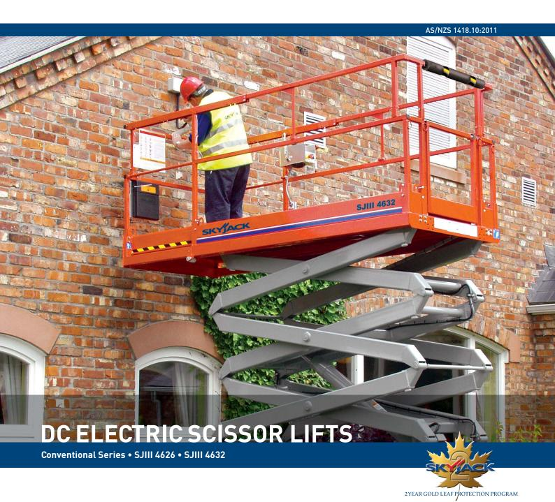
The Conventional Series DC Electric Scissor Lifts offer high capacity and large platform areas, making them suitable for any on-slab application. Featuring variable speed rear wheel hydraulic drive, the Conventional Series offers working heights up to 11.9 m and up to 30% gradeability. A standard 1.2 m roll out extension deck can be secured in multiple positions, and both models can be driven at full height.
